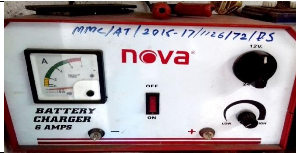
Battery charger machine Use for charging vehicle batteries
