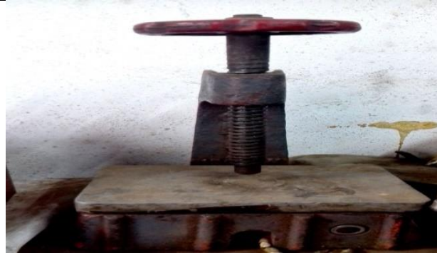
Vulcanizer Machine Use for making hot patch for tube
