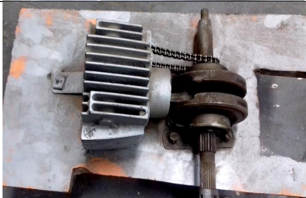
Piston with cranke shaft Working model of piston connecting rod cranke and cylinder block.
