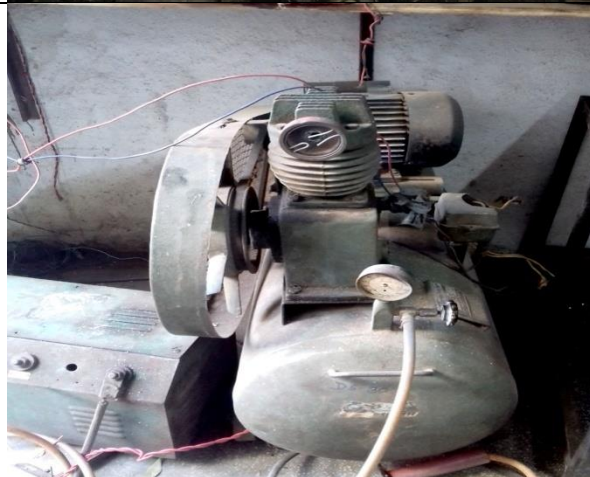
Compressor For filling air in wheel tube For cleaning Engine part like carburetor Air pressure for painting,
