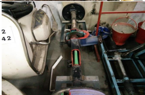
Rear axle with differential cut section model for study purpose.
